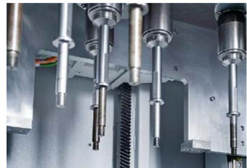
This made it clear that the DF 5 Standard would be used as a basis and that it would need to be equipped with a lot more space and much more power. The existing standard machine was redesigned to enable it to accommodate up to five workpiece holders with a minimum circumscribed circle of max. 330 mm.
