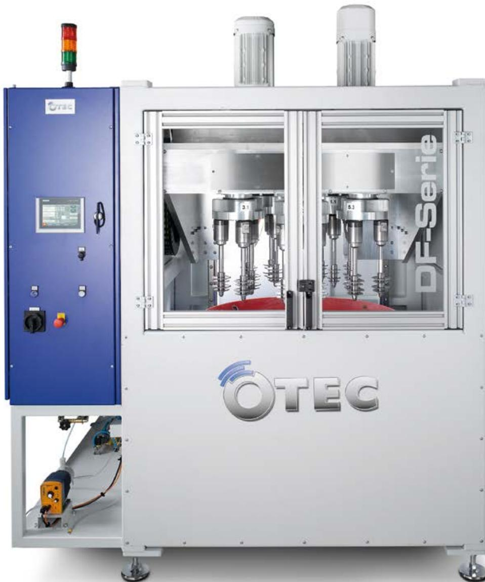
The workpiece holder has now become bigger and more adaptable, and because of the weights involved, it is compatible with the new S9 adaptor. Up to five workpiece holders with three adaptors each can be used in the new DF 5 wet/330. The machine can now accommodate tool diameters of max. 330 mm, tool weights of up to 20 kg and tool lengths of 280 mm.
