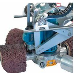
The central head carrying the tools is an extremely strong and compact unit. The gear head is mounted in an ingenious, unique scissortype suspension system.
