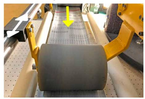
The oscillating contact wheel moves across the infeed direction pressing the grinding belt towards the workpiece.
